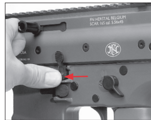
Using the bolt release as a bolt lock.
