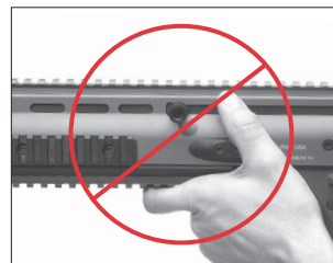
Incorrect hand placement
